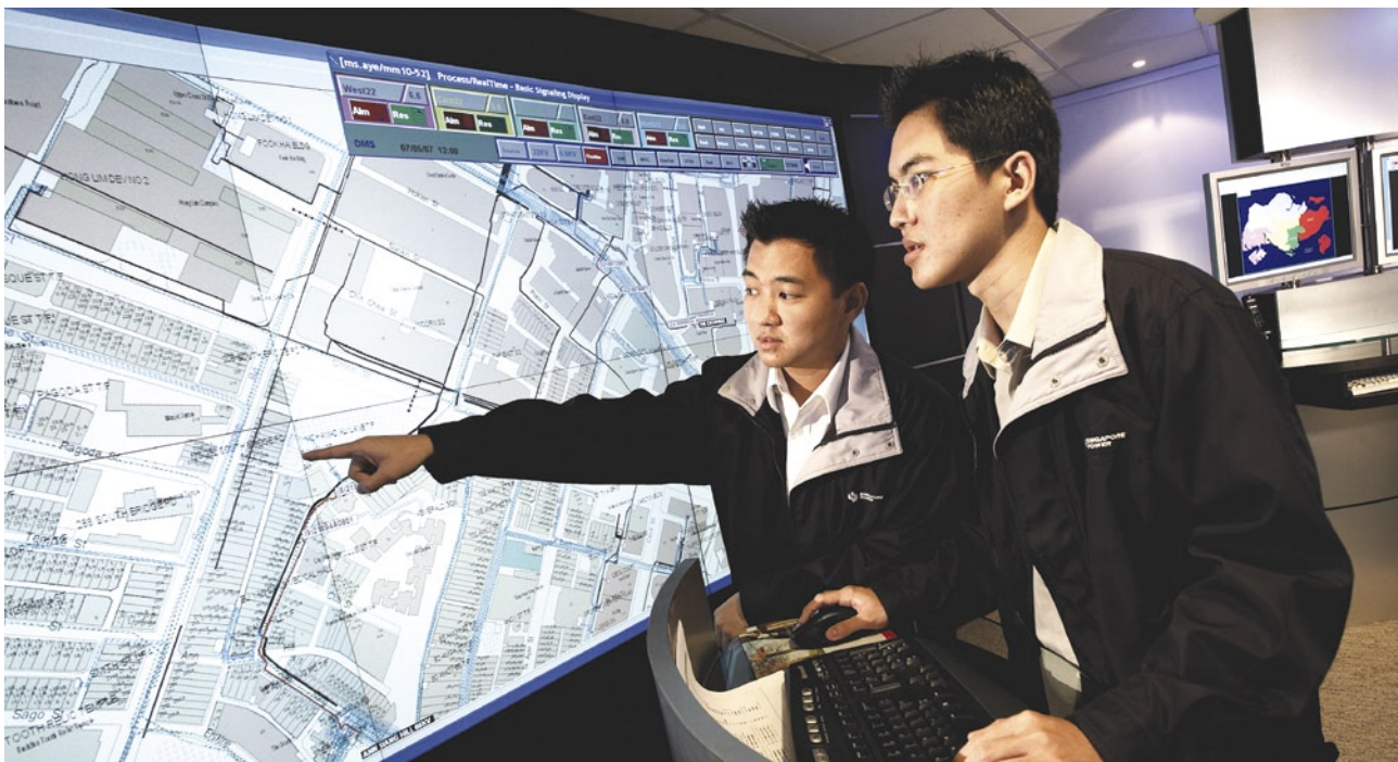
The Geographical Mapping System provides a unified view of land, electrical facilities and schematic information for SP PowerGrid's staff all over the island.
