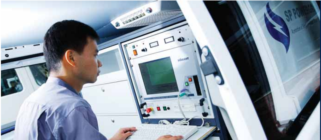
The cutting-edge Oscillating Wave Test equipment helps engineers monitor the condition of cables
