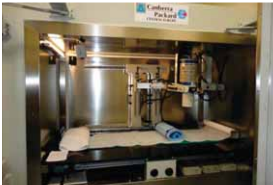
Inner View of WBC System Installed at NDCL Lab Islamabad
