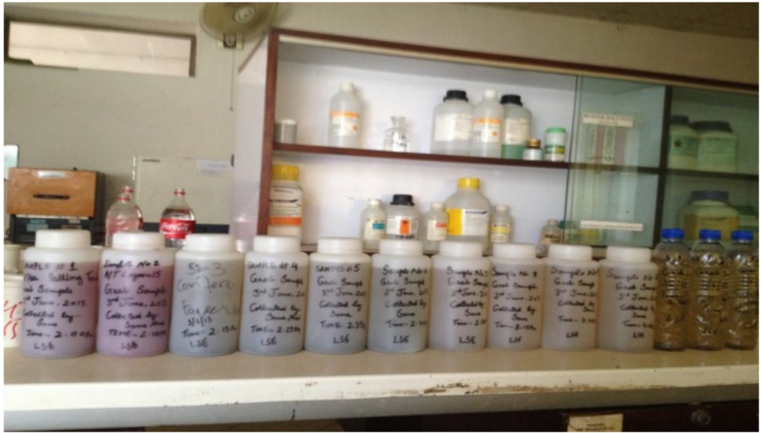
Fig.3.8: Collected tannery wastewater samples in Polyethylene bottles.
