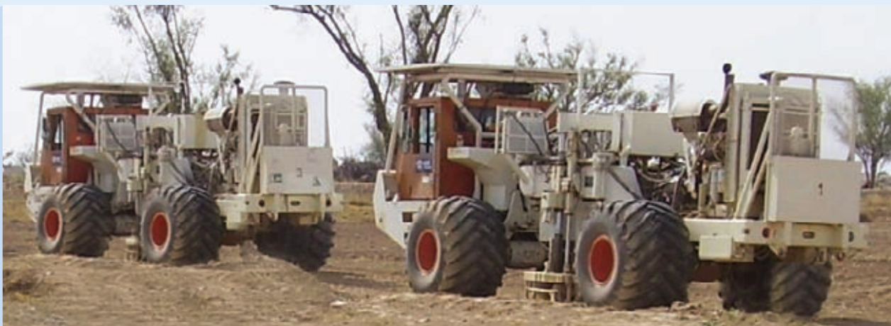
Seismic vibrators working for onshore hydrocarbon exploration.
