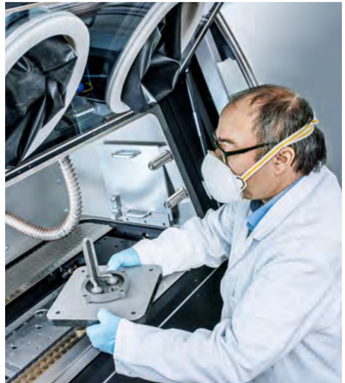
Innovative manufacturing method: Laser melting ® allows the production of highly complex metal components which are built up layer by layer.
