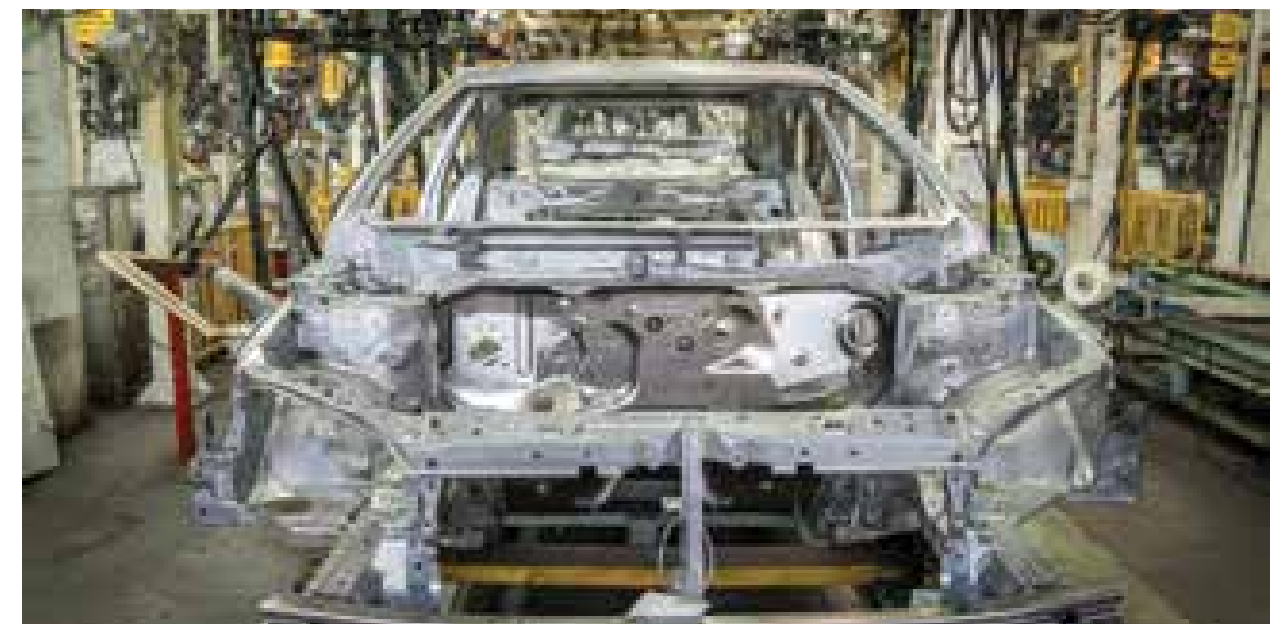
Corolla body shell with high tensile steel parts
