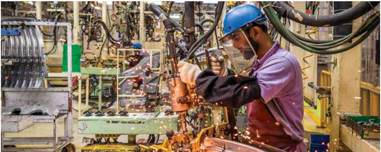
Team member welding sheet metal parts
