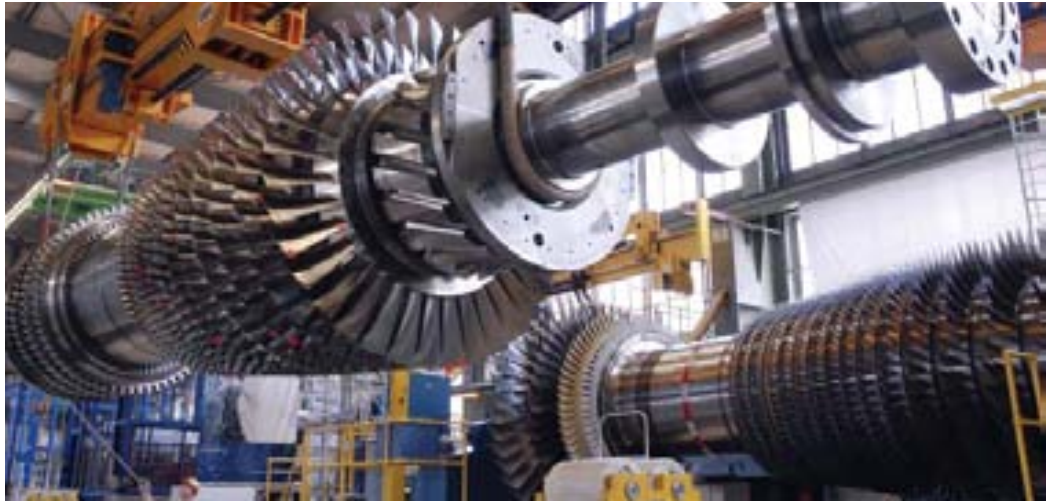
The SGT5-8000H – the largest and most powerful gas turbine in the world. After the test phase in Irsching, near Ingolstadt in Bavaria, the system will be expanded into a high-efficiency combined cycle power plant with an output of approximately 530 megawatts and efficiency of over 60 percent.
