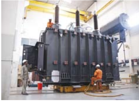
^ Power transformer - Ready for Electrical test and Customer Inspection
