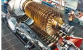
SGT6-2000E gas turbine during assembly at the Berlin plant in Germany
