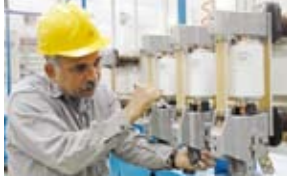
VCB shop – assembly of vacuum circuit breaker of a medium voltage panel
