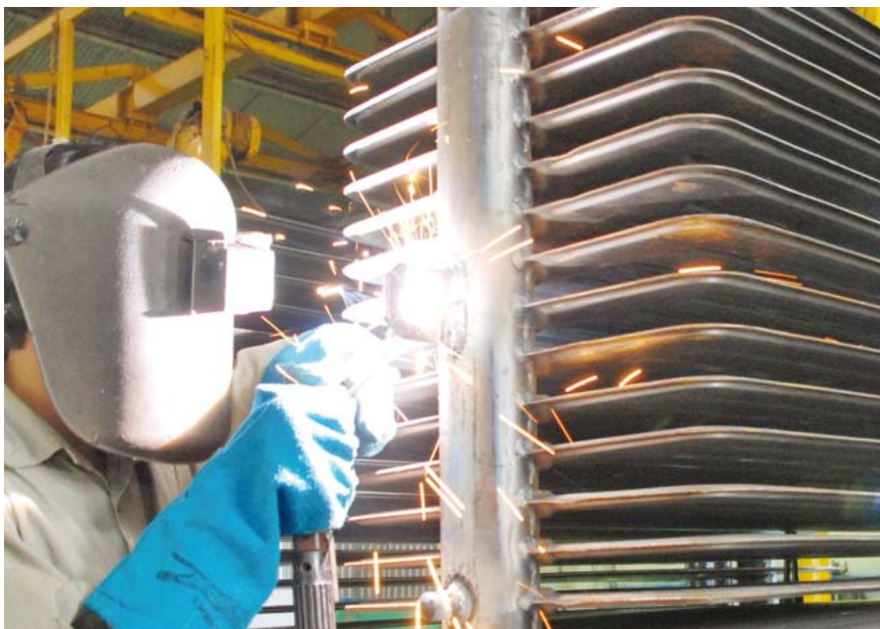
No leakages! Transformer Tank and Radiator manufacturing.
