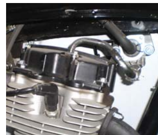
Added ASV unit for 2nd stage burning to reduce emission
