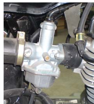
New Euro-II standard carburetor for fuel efficiency and reduction in emission
