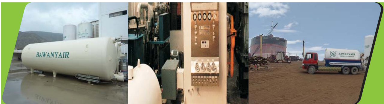
BULK LIQUID STORAGE TANK.
