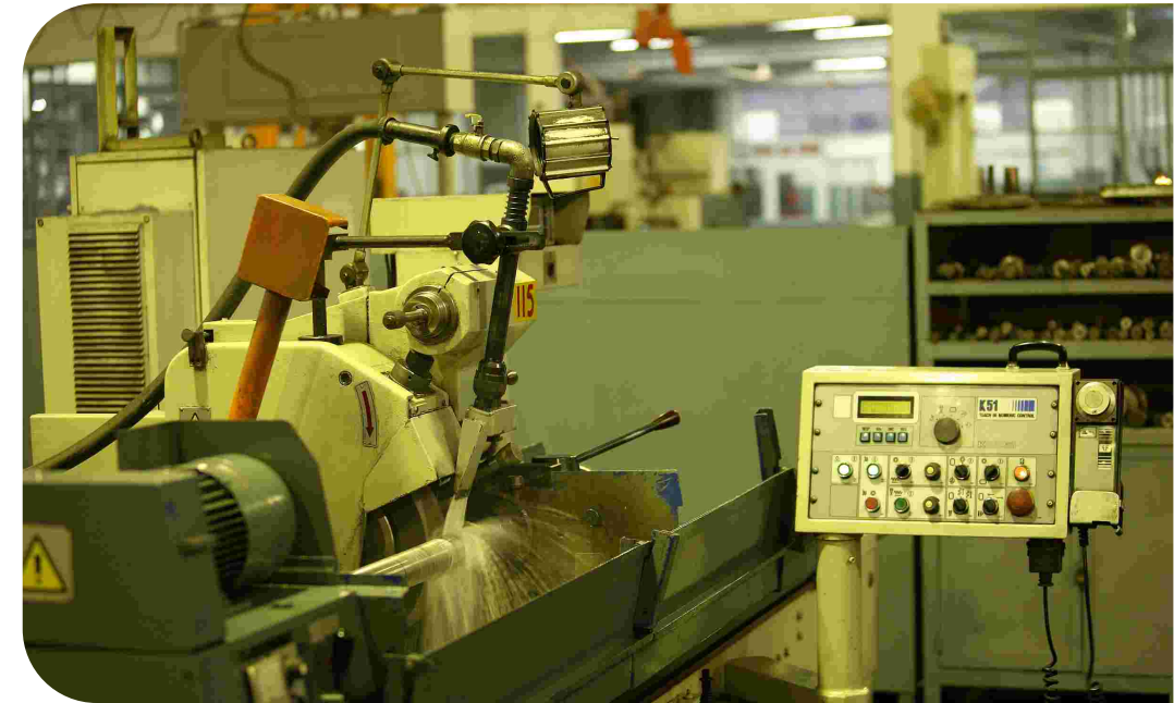
Pump shaft grinding in operation
